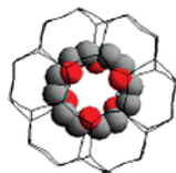
Figure 1. Eighteen-ring cage of MSO with the occluded carbon atoms (gray) and oxygen atoms (red) of the 18-crown-6 ether molecule.
